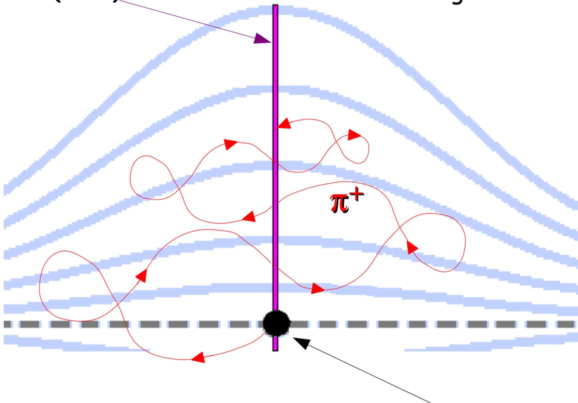
Low energy pions return to "fin" of production target (every surface is both an entrance and an exit surface). At each pass, the pion loses energy and is scattered.
