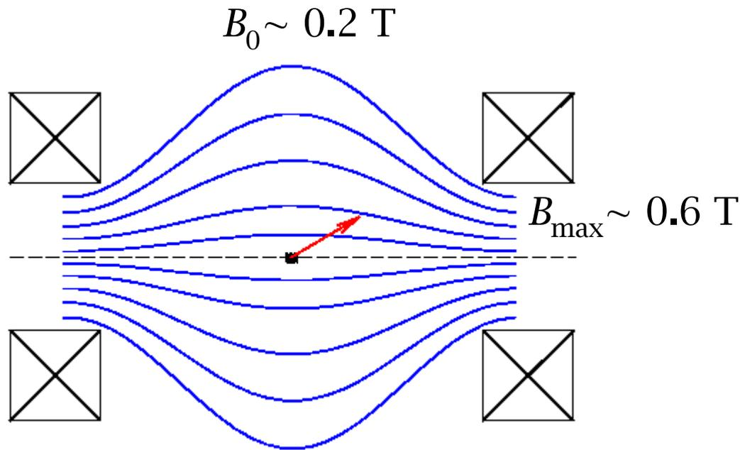
$$\theta_{\text{crit}} \sim 35^\circ \Rightarrow \Omega_{\text{escape}} \sim 1.5 \text{ sr}$$
