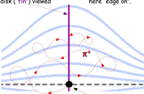
Low energy **pions return** to "fin" of <u>production target</u> (every surface is both an entrance and an exit surface). At each pass, the pion loses energy and is **scattered**.
